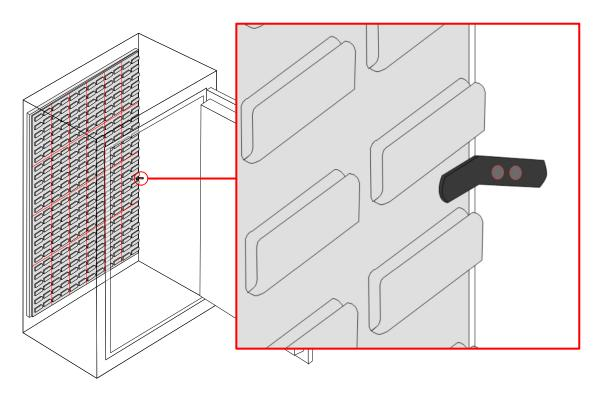
Due to the shallow nature of gun safe drywall we recommend trimming the pilot extension off of the anchors. Wire cutters work best.
